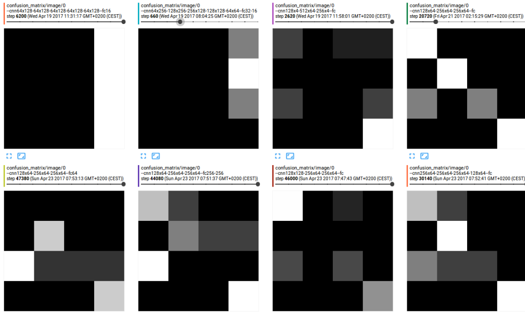
Figure 4.12: Models are monitored through the training process: during weight updates a small subset of unseen entries is inferred, and compared to the ground truth labels. In these confusion matrices the row sum represents a histogram of the labels, while the column sum would represent the histogram of the network's choice. Their intersection results in the talkative heat maps. Notice that those models whose confusion matrix is mainly diagonal is performing well, and those networks which have been collapsed gives a matrix where only a single column can be seen (i.e. first row, the two rightmost matrix).
