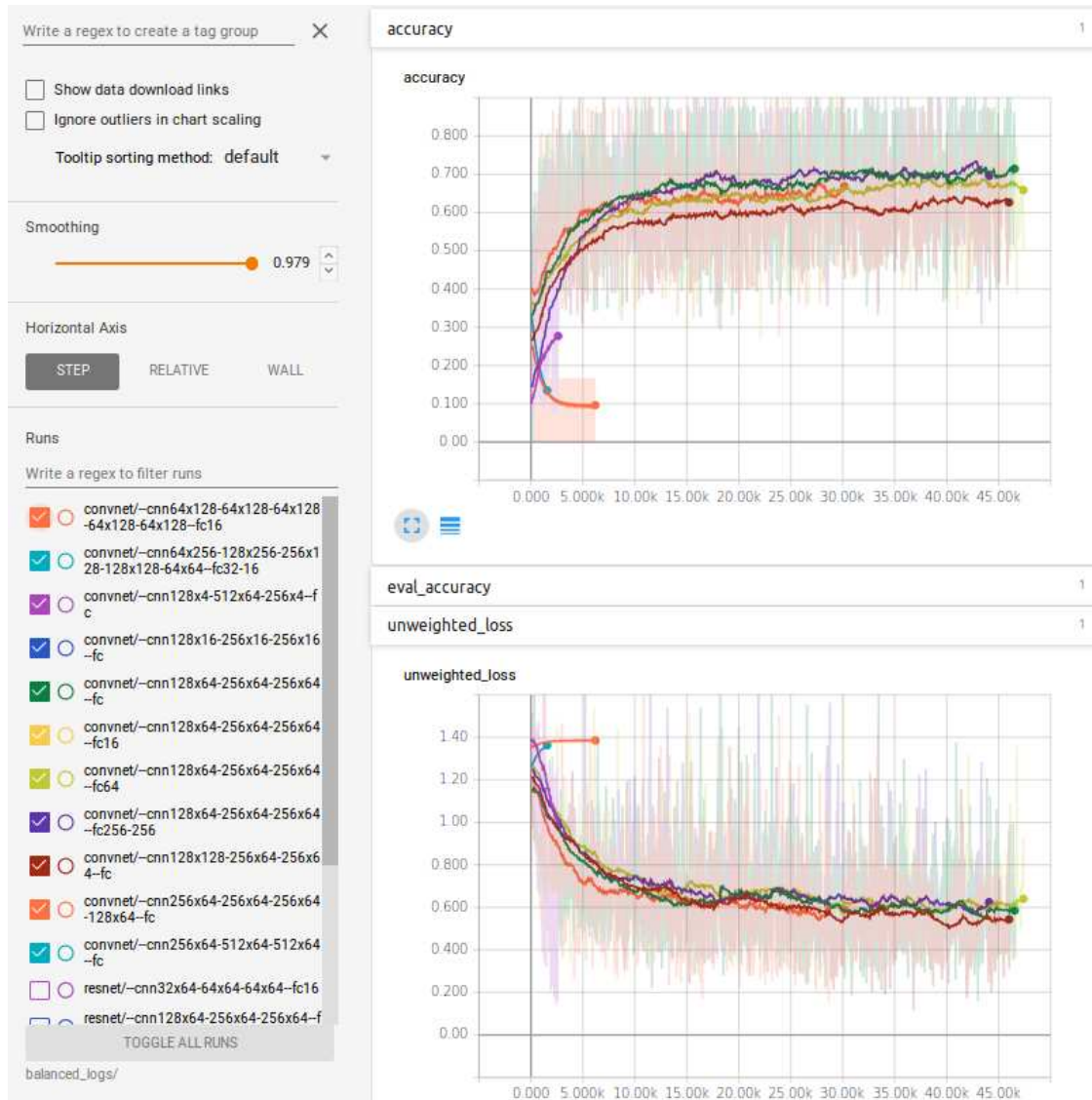
Figure 4.10: Overall performance of the FCN approaches plotted in TensorBoard. Top: Accuracy derived from the confusion operator. Bottom: Unweighted loss during training
