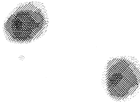
Fig. 2 Proton nuclear magnetic resonance zeugmatogram of the object described in the text, using four relative orientations of object and gradients as diagrammed in Fig. 1.
