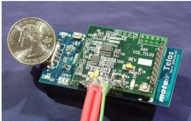
Telos wireless platform with intelligent signal processing daughtercard ISPM
