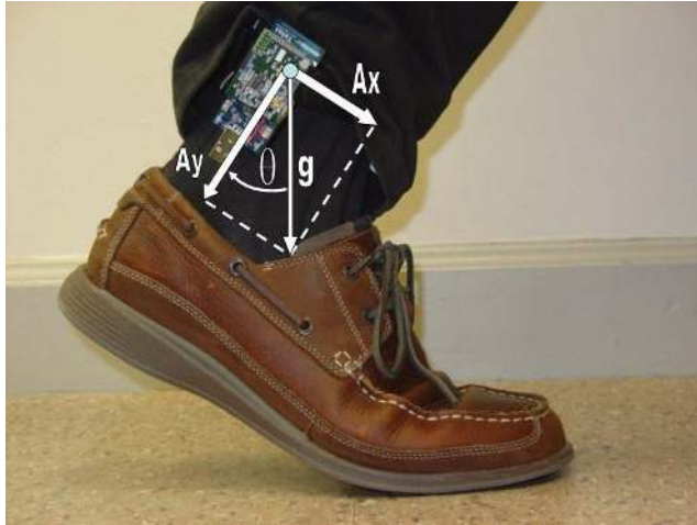
Activity sensor on an ankle with symbolic representation of acceleration components
