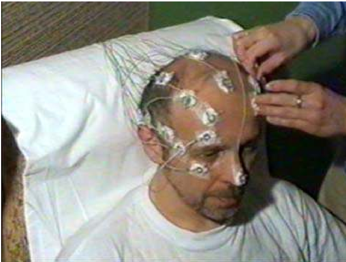
Fig. 5. Scalp EEG electrodes, individually attached by glue strips. Reference electrode on the nose. EOG electrodes above and below the eyes and at the outer canthus of the right eye.
