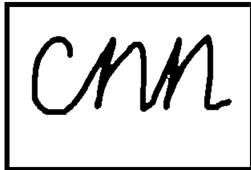
output of EROSION operation
