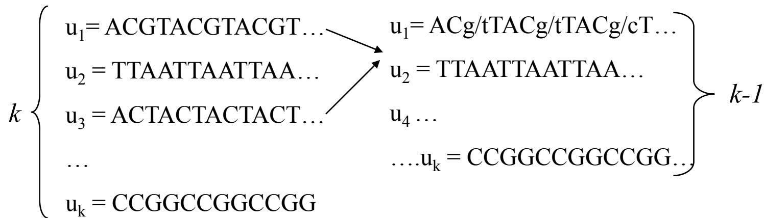
Sequences  $u_1$  and  $u_3$  are combined into a profile and replaced.
