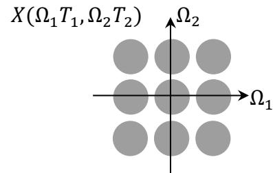
The spectrum of the digital image is periodic. The sampling periods  $T_1$  and  $T_2$  controls:
